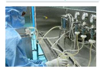
State of the art instrumentation and monitoring equipment coupled with flexible simulation jigs are used to achieve near perfect simulation of worst case process condition, an essential pre-requisite to filter validation with specific drug products.
